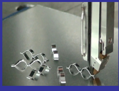
Ribbon bonding (W:2mm, t:0.2mm)
