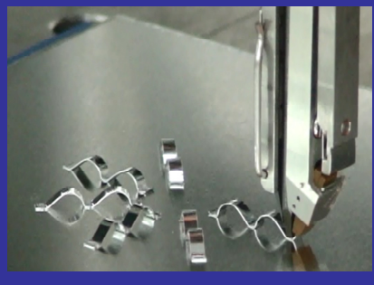
Ribbon bonding (W:2mm, t:0.2mm)
